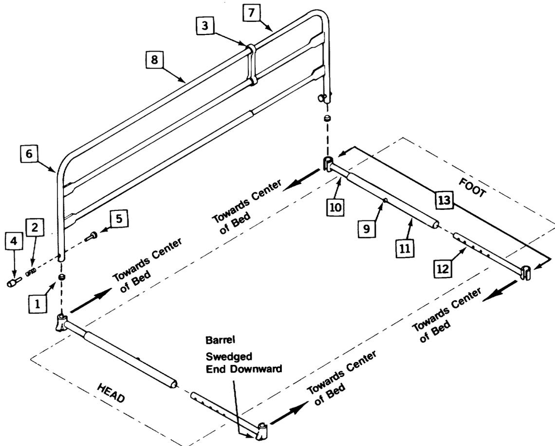
FIGURE 1 - INSTALLATION OF HOMEBED RAIL MODEL NO. 6631
