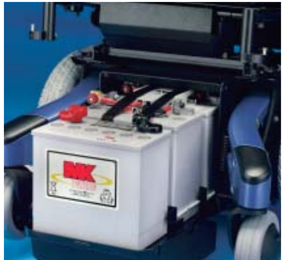
New door, tray and harness are all that is needed to house the ventilator battery.
