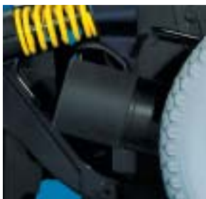
2-pole motors offer true free-wheeling with a clutch release.
