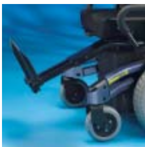
Allows for in-the-field knee angle adjustment from 90° to 60°.
