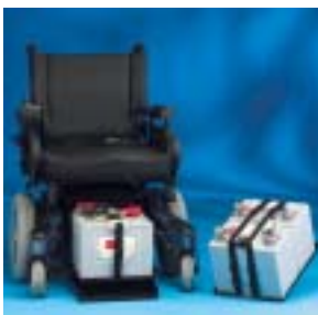
The wiring harness of the TDX will work with MK batteries or those with this configuration.
