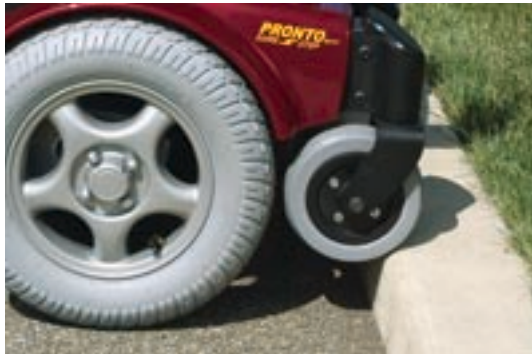
Front casters automatically lift up to accommodate transitions up to three-inches for a smooth and controllable ride.
