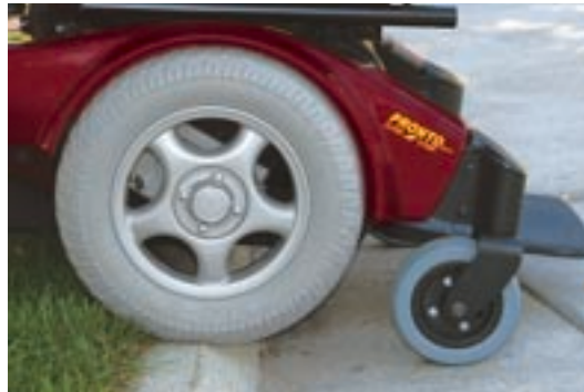
SureStep design flexes to maintain drive-wheel traction while driving over transitions.
