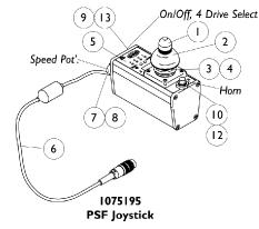
STANDARD: This PSR joystick includes a toggle on/off combined with a drive select and a push button horn. No speed selector. PBOD: This PSR joystick includes push button on/off with a push button drive select. This gives you access to the four drives, but no horn and no speed select.
