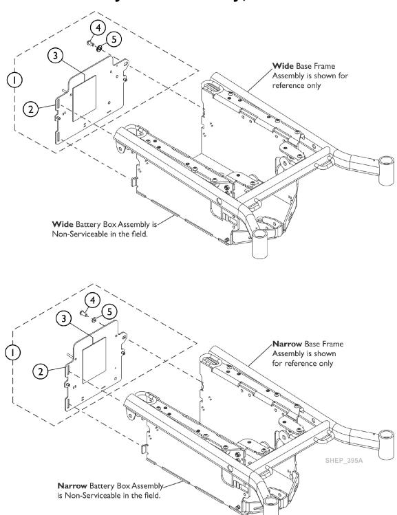
**Battery Box Assembly, Rear Plate**
