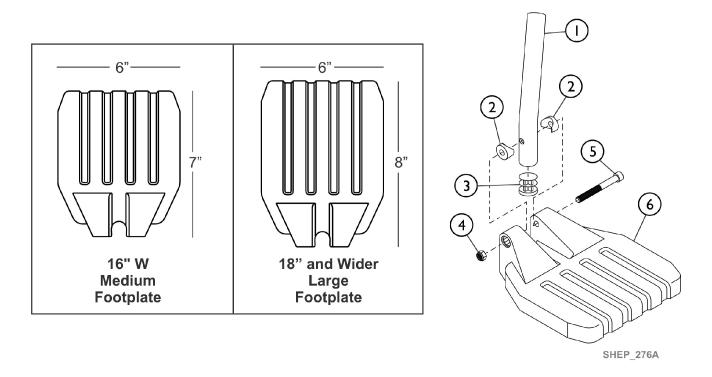
Pivot/Slide Tube and 1651 Composite Footplates
