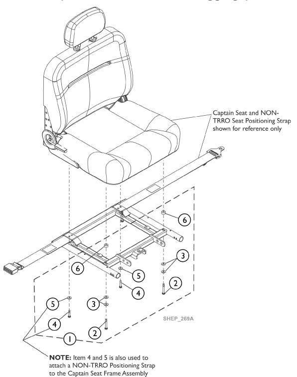
Captain Seat Assembly Mounting Hardware - Non-Elevate & (Elevate w/ CTMT Front Riggings)
