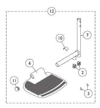
Front Riggings - Pivot/Slide Tube w/ Footplate
