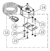
4-Way Switch Quad Link Mounting Hardware Before 10/31/05
