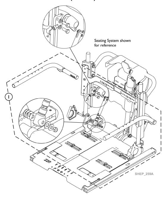
Reclining Arm Assembly, Flip Back, Adjustable Height, Curved, Reduced Extension (12-1/2-16" H) MXFB-C
