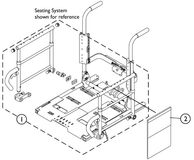
Dual Post Arm Assembly, Quick Height Adjust, Reduced Extension (Pair) (15-3/4-18-3/4'' H) ADPAH-T
