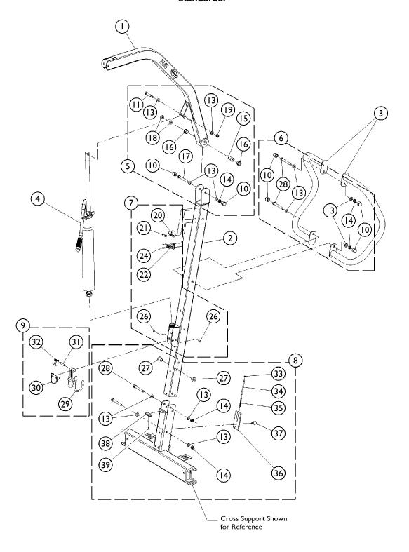
Hydraulic Lift - Mast / Boom Assembly
