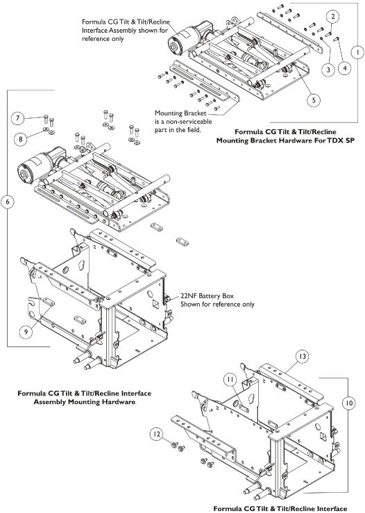
Mounting Plate Attaching Hardware
