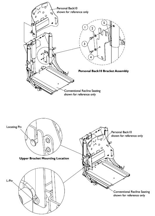
Lower Bracket w/ L-Pin Mounting Location
