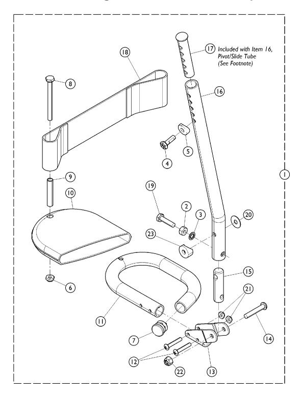
Pivot Tube w/ Footplate Assembly - Tubular w/ Attaching Hardware and Heel Loops
