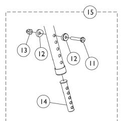
Slide Tube Mounting Hardware for 1651 Composite Footplates
