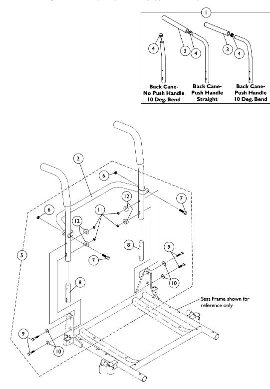
Back Canes, Spreader Bars and Attaching Hardware NOTE: Chairs manufactured with a seat width, seat depth or back height of 20" and greater including all user weight selections (U400) will be equipped with a spreader bar standard.
