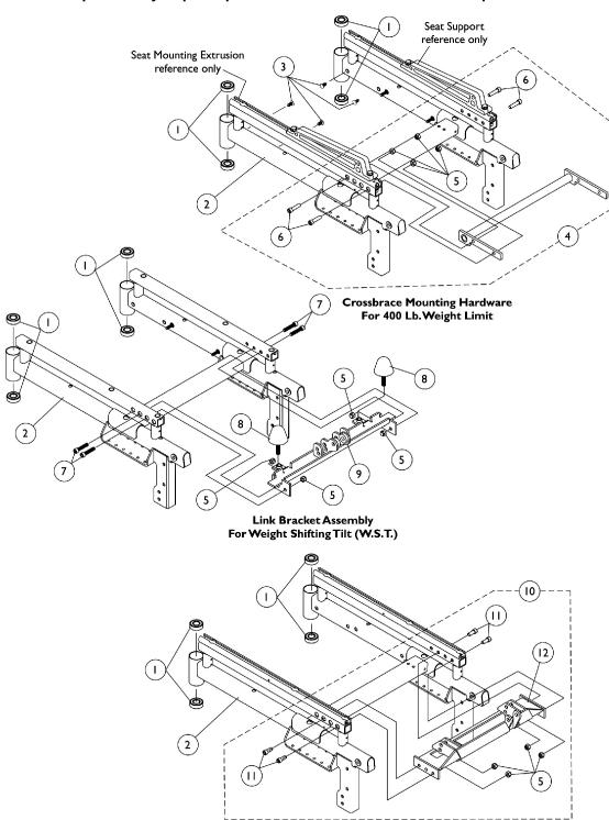
Front Support Bracket Hardware For Power Tilt Only (PTO)
