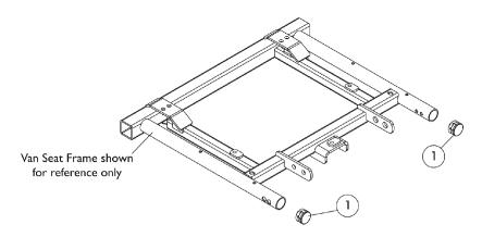
Swingaway Front Rigging Non-Hanger Hardware (When Front Rigging Is Excluded From Chair) Or When Center Mount Riggings are used
