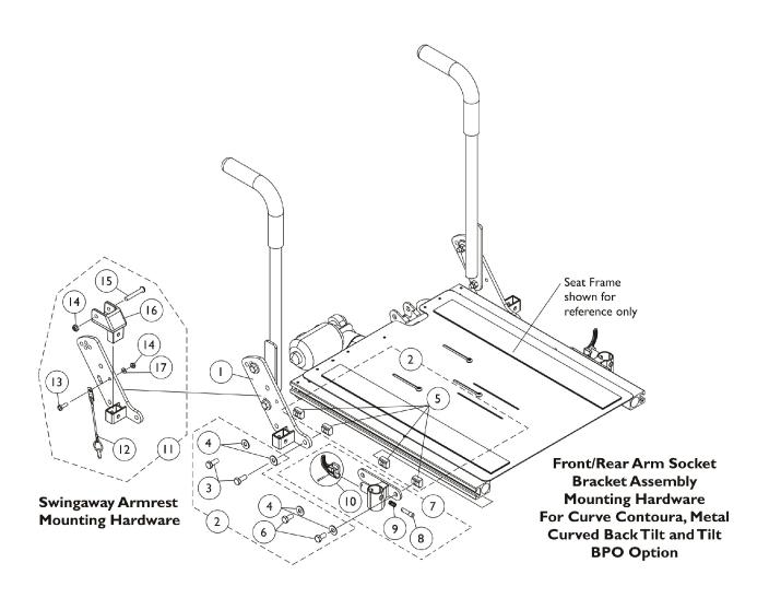
Arm Mounting Hardware CGT/CGTE (12" - 16" W x 16" - 18" D) and (16" - 22" W)
