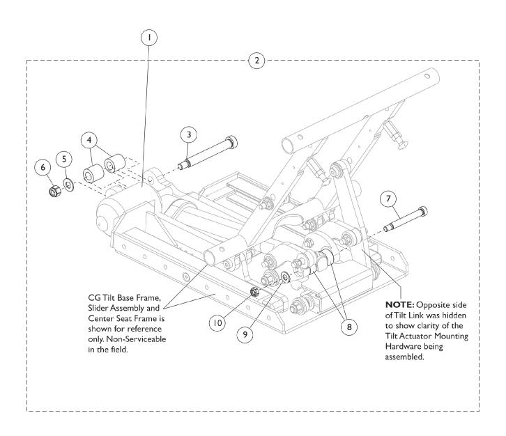
Tilt Actuator Motor (Conventional) and Mounting Hardware
