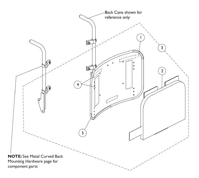
NOTE: Curved Back mounts only to back canes without a 10 degree bend. NOTE: As of 8/15/08 the Curved Back material changed from ABS Plastic to Metal as inventory runs out. You must ask the customer if they have an ABS Plastic or the Metal Curved Back model when replacing components. All service replacement Back Assemblies with Hardware shipped will be metal. New Headrest Mounting Hardware is required when replacing an ABS Curved Back with a Metal Curved Back.
