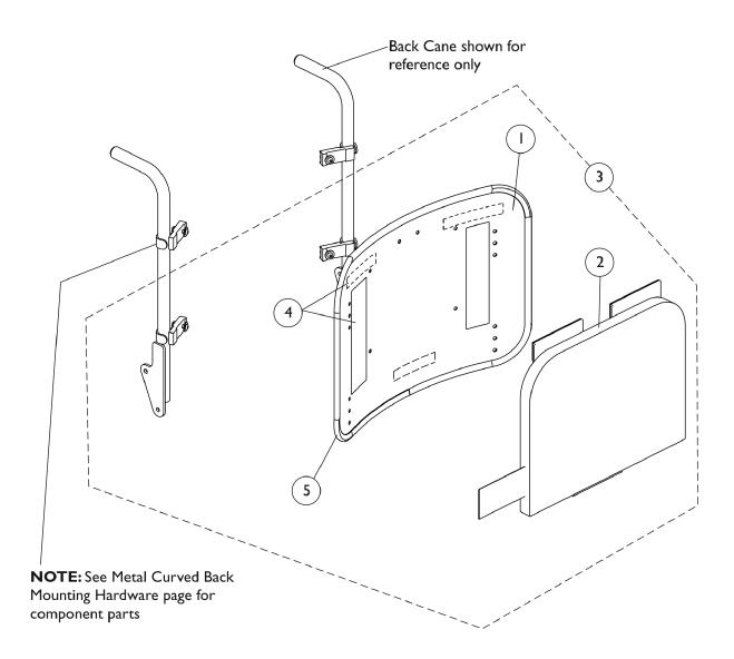
NOTE: Curved Back mounts only to back canes without a 10 degree bend. NOTE: As of 8/15/08 the Curved Back material changed from ABS Plastic to Metal as inventory runs out. You must ask the customer if they have an ABS Plastic or the Metal Curved Back model when replacing components. All service replacement Back Assemblies with Hardware shipped will be metal. New Headrest Mounting Hardware is required when replacing an ABS Plastic Curved Back with a Metal Curved
