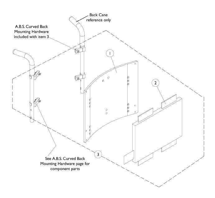
NOTE: ABS curved back mounts to back canes without a 10 degree bend.
