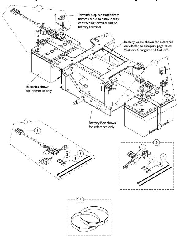
**Battery Wire Harnesses and Battery Straps**
