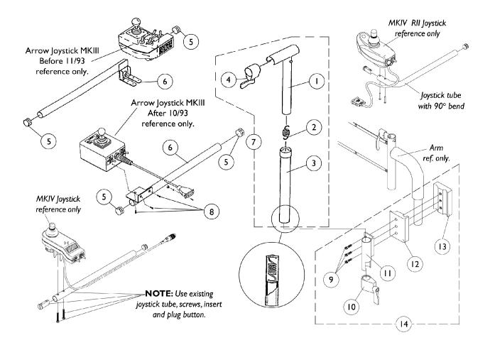
**Mid-Line Swing Bracket Assembly** NOTE: Joystick tube with 90 degree bend replaces the standard tube when joysticks PSF, PSR and (RII part number 1092610) are used. Joystick Tube with 90 degree bend must be ordered as a special when a replacement is needed.
