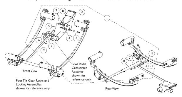
Right Side Foot Pedal Tilt Release Assembly
