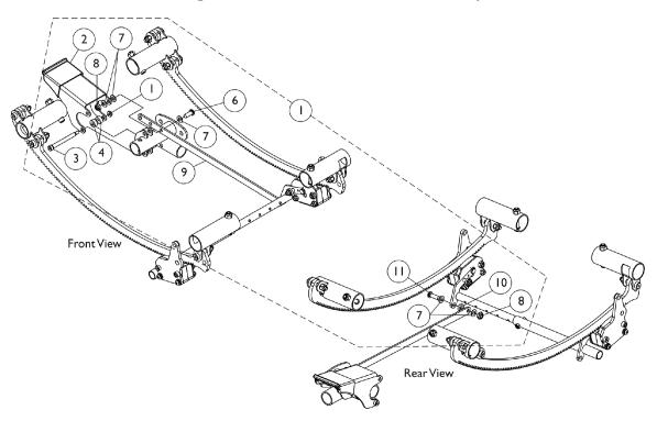
Left Side Foot Pedal Tilt Release Assembly
