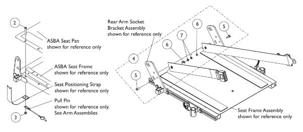
Seat Positioning Strap Mounting Hardware (For ASBA Seating) Seat Positioning Strap Mounting Hardware (For ADJASBA Seating)
