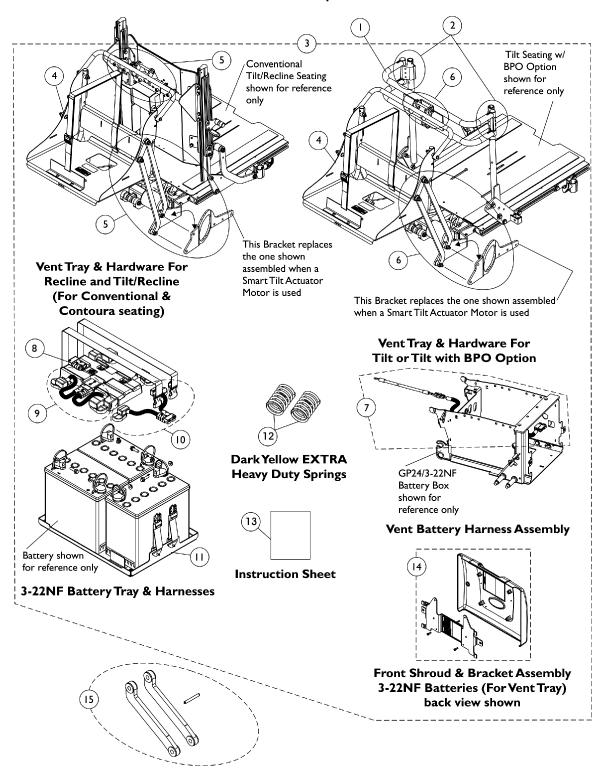
NOTE: Please read all footnotes before ordering a Vent Tray Kit, additional components may be required. TDX SR models always use SMART Actuators. Vent Tray is excluded from TDX SP/SR model wheelchairs with TRRO option
