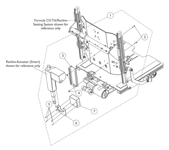
Mk6i Recline Integrated Actuator Module (RIAM) and Mounting Hardware
