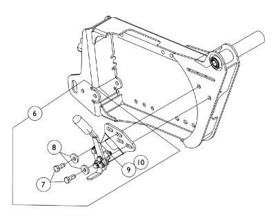
Wheel Lock Assembly introduced on I/I/06 to be used for TTHD TrueTrack <u>Heavy Duty</u> GB motors.
