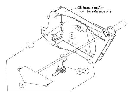
Wheel Lock Assembly for Non-Heavy Duty GB motors offered On-Chair thru 1/25/04. After 1/25/04 TTHD TrueTrack Heavy Duty GB motors became the only On-Chair GB motor choice. Due to wheel lock interference with the brake lever, wheel lock assemblies were not offered On-Chair for Heavy Duty GB motors until 1/1/06. See wheel locks shown below.
