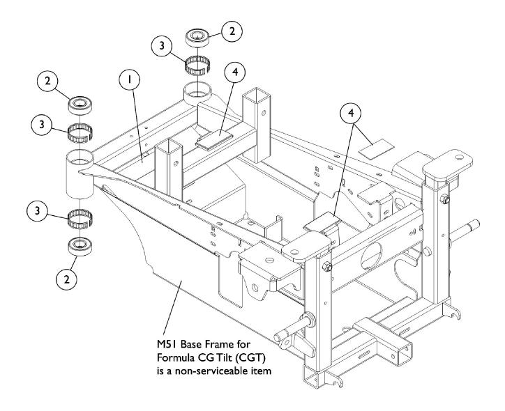
Base Frame, Bearings, & Hardware Refer to parts catalog "Pronto M50/M51 with SureStep After 1/19/05 and Pronto M61 with SureStep" Form # 04-050 for the M51 Base Frame mounted components such as casters, forks, drive wheels and
