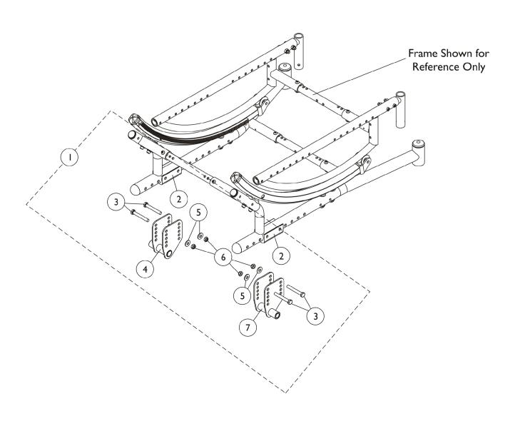
Axles, Axle Mtg. Plates & Hdwr - Chairs w/Vent Tray
