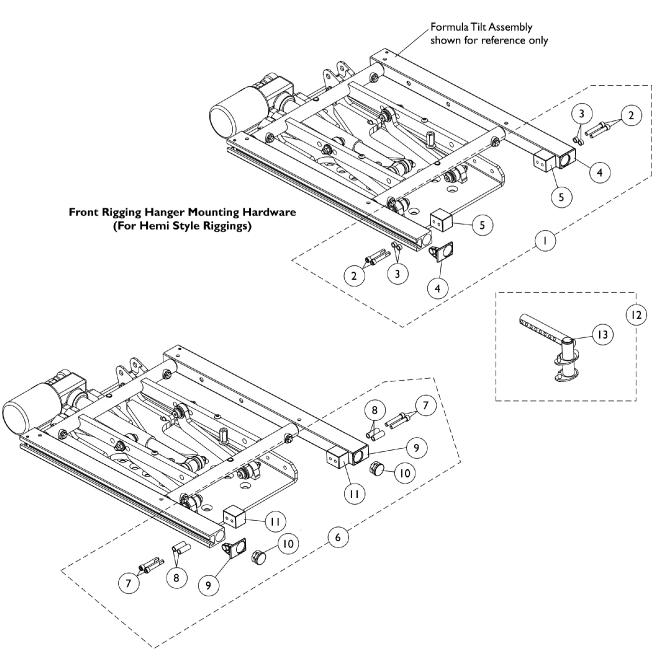
Front Rigging Non-Hanger Hardware (When Front Rigging is Excluded From Chair)
