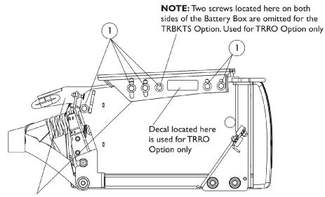
**NOTE:** The Seat Frame Mounting Plate and Battery Box Tie-Down Bracket use the same mounting hardware
