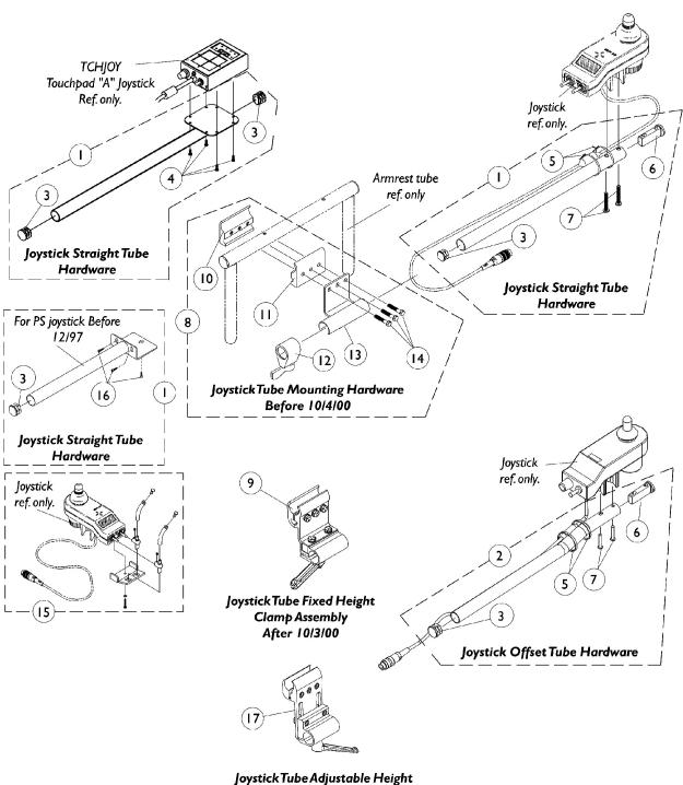
Joystick Tube Adjustable Height Clamp Assembly
