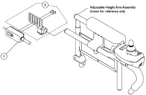
Toggle Switch Joystick Tube Mounting Hardware
