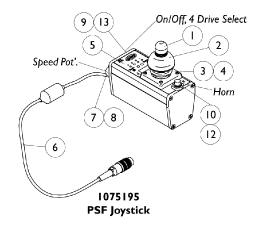
\*\*\* STANDARD: This PSR joystick includes a toggle on/off combined with a drive select and a push button horn.
