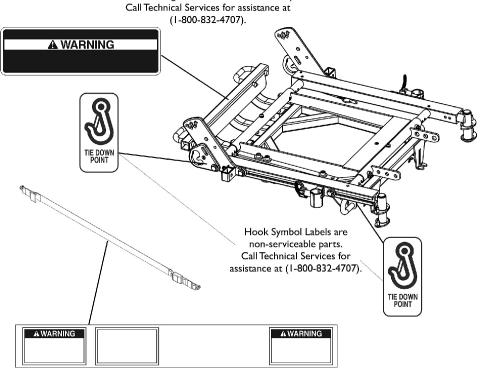
Occupant restraint pelvic belt comforms with ANSI/RESNA. WC/19 Warning Label is sewn onto the pelvic belt assembly.
