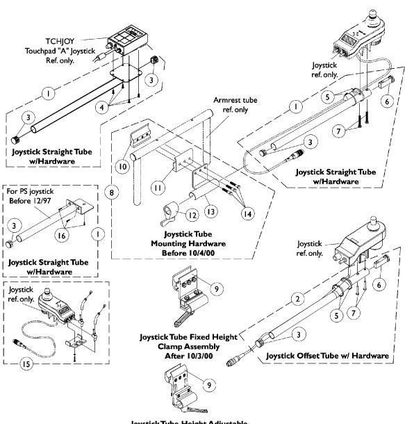
Joystick Tube Height Adjustable Clamp Assembly (ARM250)
