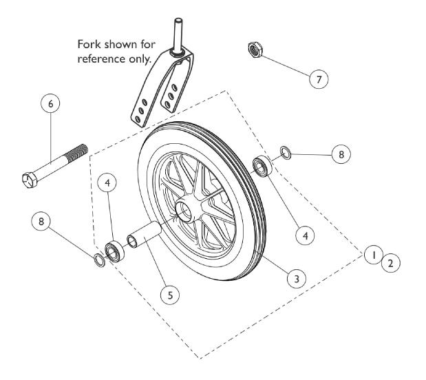
Casters and Mounting Hardware NOTE: If your chair was built with a serial # starting with "03H" or "03I", please contact an Invacare Parts Specialist for replacement parts at 1-800-333-6900 Ext. 3722.
