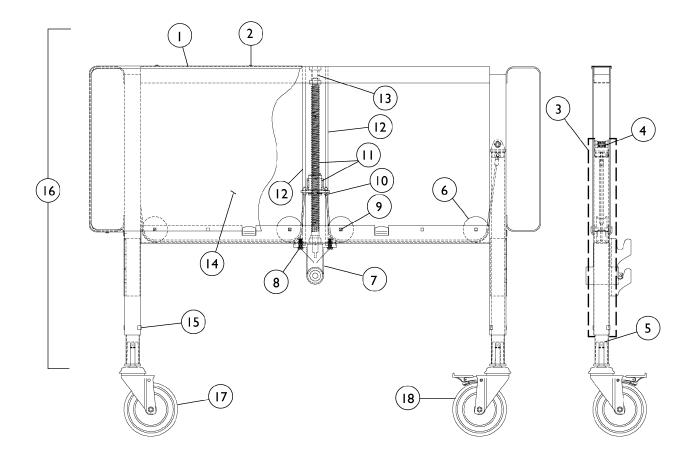
**Bed Ends - Full Electric (BAR5401)** NOTE: Bed Ends with the "Woodgrain" finish are from the BAR600 group Manufactured "before 5/05." Bed Ends with the "Composite" finish are from the BAR600IVC group manufactured "after 2/05." Please check before ordering service parts.
