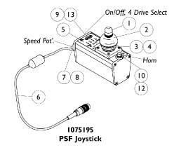
STANDARD: This PSR joystick includes a toggle on/off combined with a drive select and a push button horn. No speed selector.
