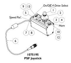
STANDARD: This PSR joystick includes a toggle on/off combined with a drive select and a push button horn. No speed selector.
