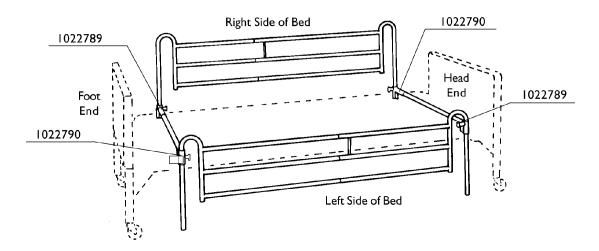
**NOTE:** To determine which crossbrace assembly, channel with barrel, or barrel only, to order, we have listed them as (1022789) Left Head End / Right Foot End or (1022790) Right Head End / Left Foot End. When the barrels are used on the opposite side of the bed, the parts are reversed.
