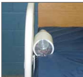
Zone 3 Between the Rail and Mattress
