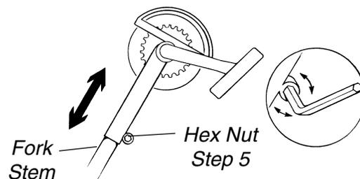
FIGURE 2 - EXCELERATOR/LI'L EXCELERATOR HAND CRANK ASSEMBLY INSTALLATION
