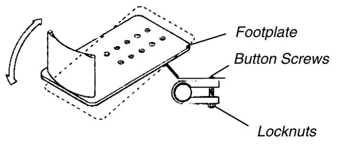
**FIGURE 1 - FOOTREST ADJUSTMENT/REPLACEMENT**
