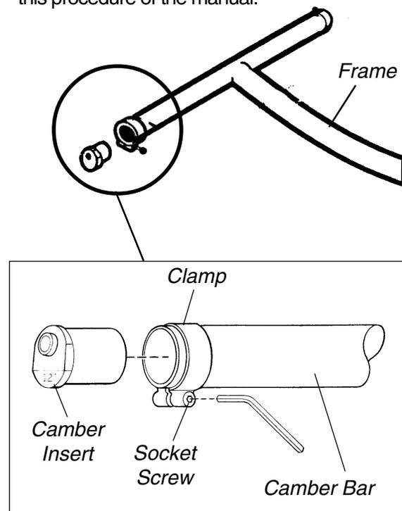
FIGURE 4 - REPLACING CAMBER INSERTS
