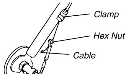
FIGURE 2 - LI'L EXCELERATOR THREE (3) SPEED SHIFTER CABLE ADJUSTMENT
