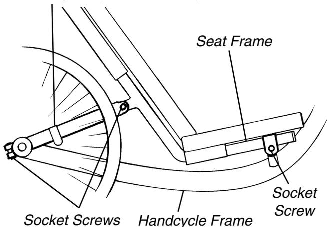
**FIGURE 3 - SLIDING SEAT ADJUSTMENT - EXCELERATOR XLT/XLT 2000**
