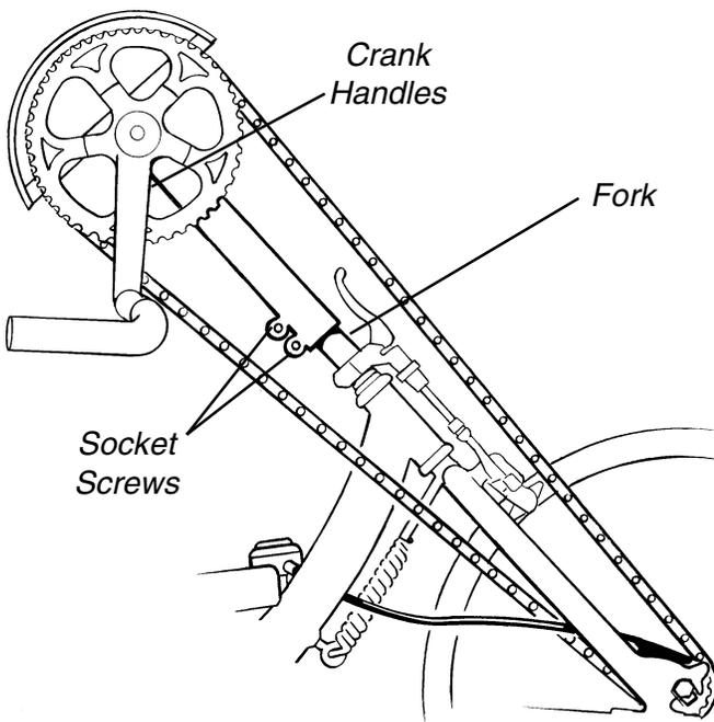
FIGURE 3 - EXCELERATOR - XLT CHAIN ADJUSTMENT
