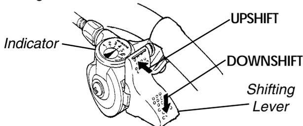
**FIGURE 1 - SHIFTING GEARS - EXCELERATOR/EXCELERATOR XLT (SEVEN [7] SPEED)**
