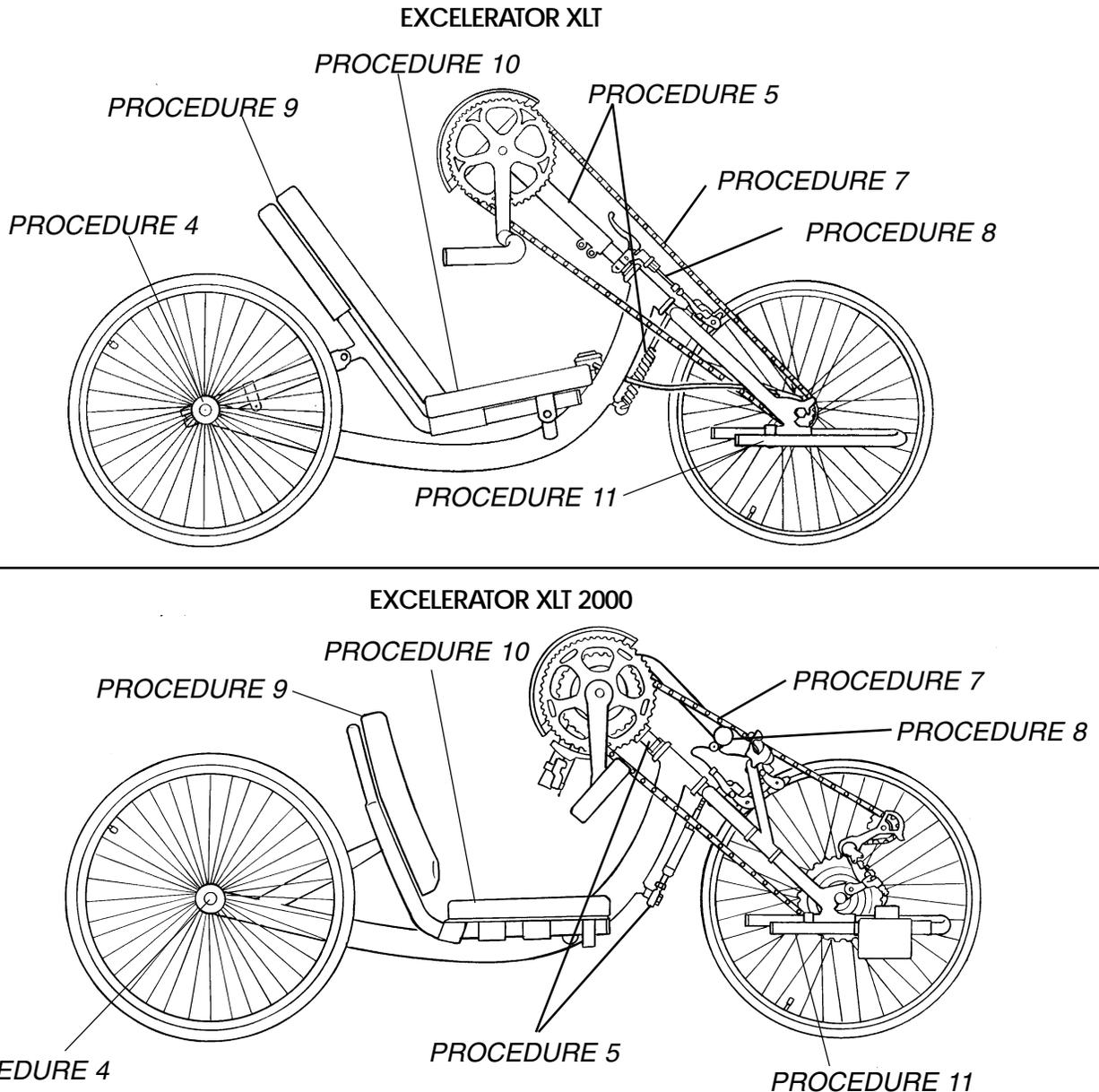
FIGURE 2 - EXCELERATOR XLT/XLT 2000 ASSEMBLY PROCEDURES
