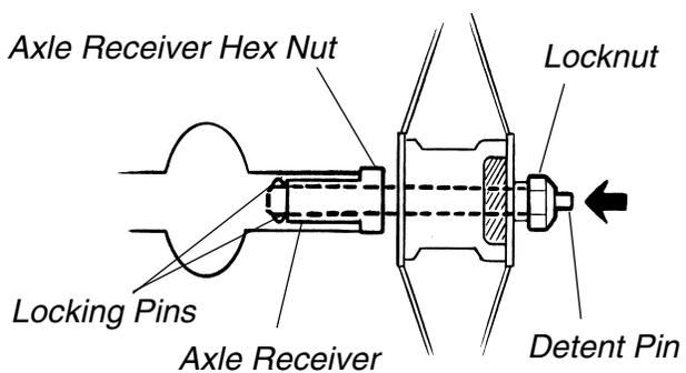
**FIGURE 1 - INSTALLING/ADJUSTING THE REAR WHEEL AND QUICK-RELEASE AXLES**
