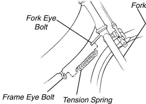
FIGURE 4 - TENSION SPRING REPLACEMENT/ADJUSTMENT
