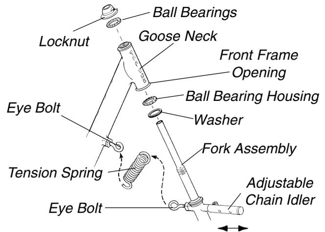
FIGURE 1 - EXCELERATOR/LI'L EXCELERATOR FORK ASSEMBLY/TENSION SPRING INSTALLATION
