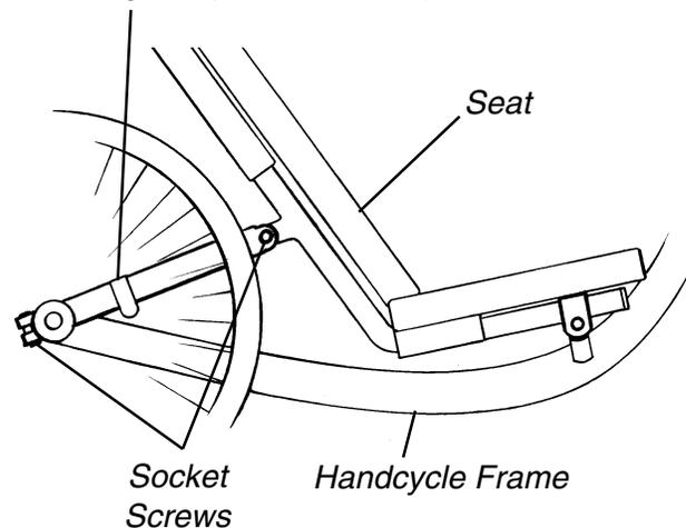
**FIGURE 4 - EXCELERATOR XLT/XLT 2000 BACK ANGLE ADJUSTMENT**
