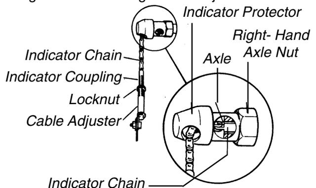
FIGURE 3 - LI'L EXCELERATOR THREE (3) SPEED INDICATOR CHAIN ADJUSTMENT
